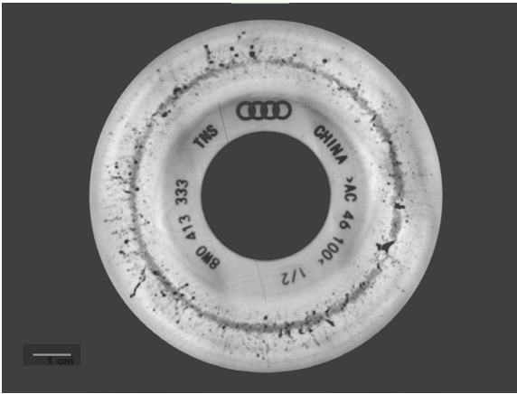
A typical cross-sectional image, contrasted to highlight pores and possible cracks.
