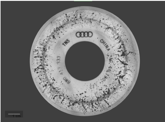
An example of a "thick-slab mode" image highlighting flaws across multiple slices, easing and fast-tracking flaw detection – the image to the right shows the "slab thickness" in a side view.
