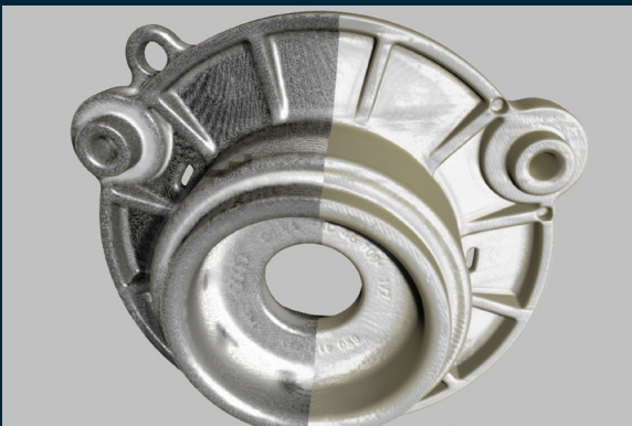
Mesh generation of the actual part geometry for simplified output.
